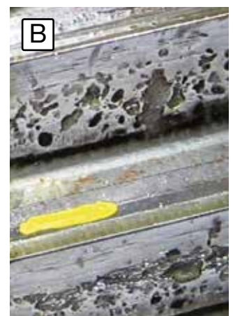
Photo B: Evident smoothing 5 months after changing to Eco Gear 460 M
